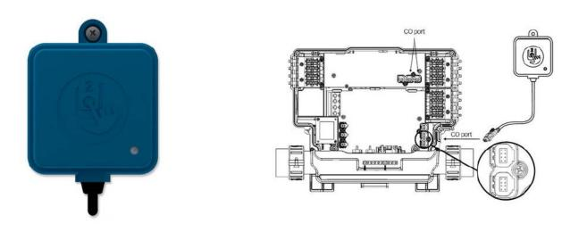
The in. touch 2 spa transmitter must be installed under the spa skirt, at least 12" (30 cm) away from any metal component or structure, as close as possible to the house to optimize the signal strength.
