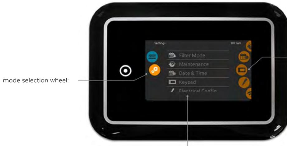
To select an item, slide the right wheel until the desired icon is highlighted in the middle or press on the menu name.
