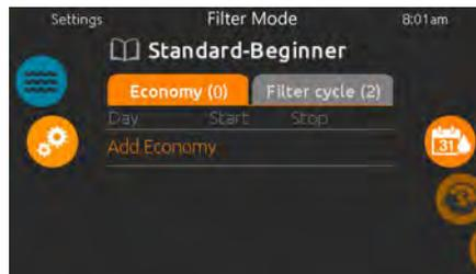
*\*In economy mode, the set point will be reduced by 20°F - which means the heating system will not be engaged unless the temperature falls to 20°F below the hot tub's set temperature.*
